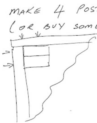
MAKE 4 POSTS FROM DOUBLE LENGTHS OF FRAMING (OR BUY SOME LENGTHS OF SQUARE CUT POSTS).. HEIGHT WILL VARY DEPENDING ON TYPE/SIZE OF KEGS + CONNECTORS, WE SETTLED ON 35" / FOR PINLOCK LORNY KEGS FIT POSTS TO INSIDE OF FRAMES TOP + BOTTOM. WITH SCREWS AT ↑'S
